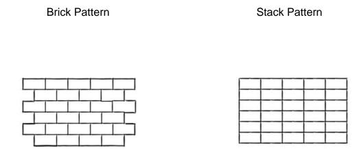
Begin to nail and glue the tiles or interlock panels to the wall making sure to follow the level lines both horizontally and vertically. Start from the middle of the wall and work your way out toward the top/bottom and left/right sides. Make sure that you adjust each tile to keep as close as possible to the level line as you go.
